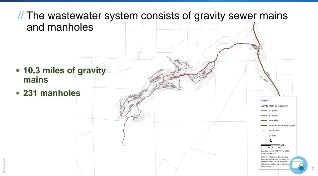
// The gravity sewer mains are mainly 6 inches in diameter
